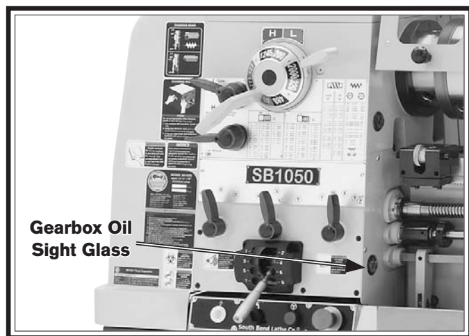
Figure 101. Location of quick-change gearbox oil sight glass.
